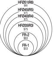
FR-1: Dia 14mm FR-2: Dia 21mm HFØ35(R3): Dia 31mm HFØ40(R4): Dia 36mm HFØ45(R5): Dia 40mm HFØ51(R6): Dia 47mm
